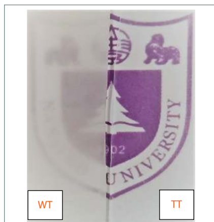
Fig. 1 Transparency of the frozen stretched states of two TSMGs at the room temperature, with separate copolymer compositions of WT (SA:DMAA = 1:1) and TT (SA:DMAA = 0.75:1).
